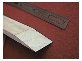
is then cut using a belt sander, file or any other means of going from 1/4" thick to a knife edge over the 1.375 distance to the mark.
